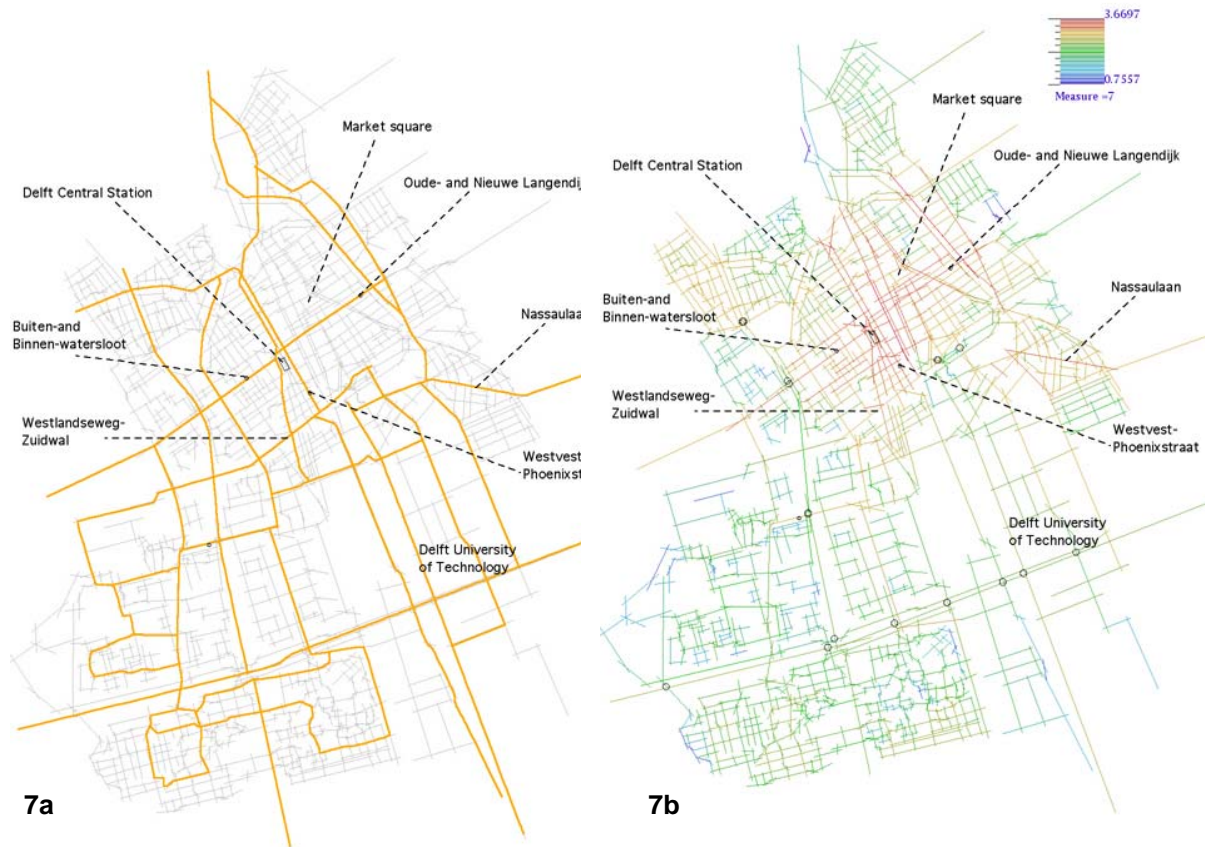
Figure 7. a) City scale movement network with the new master plan, represented by the thick orange lines; b) Area integration analysis of Delft with the New Master Plan
